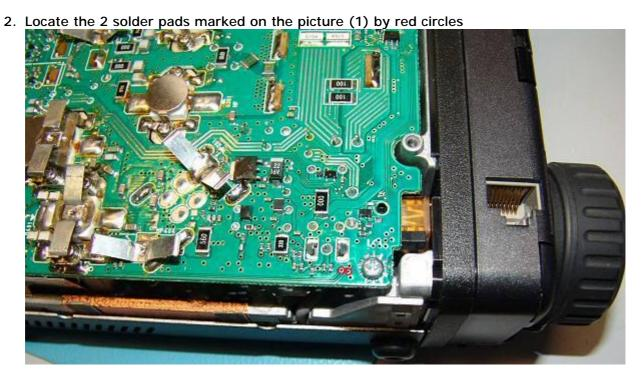
3. Clean the pads, and pre-tin them, solder the resistor to the pads
